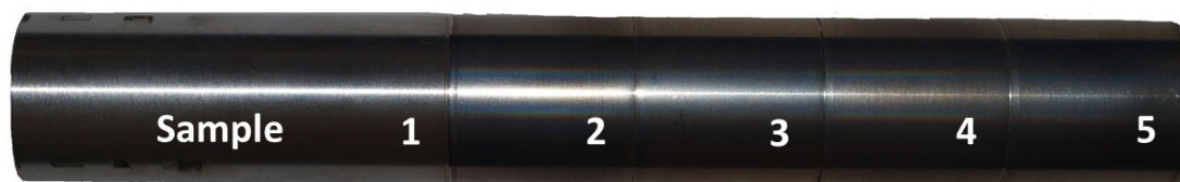
Fig. 1. Test sample from aluminium alloy with single variants of machining
